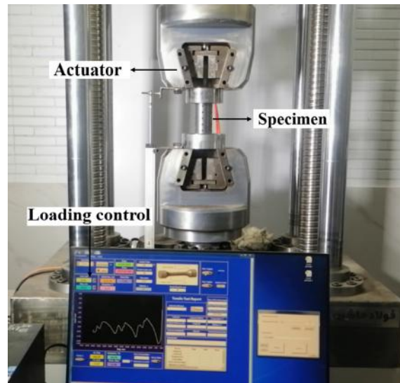
Figure 4: FOLAD MACHINE Hydraulic Testing Machine
